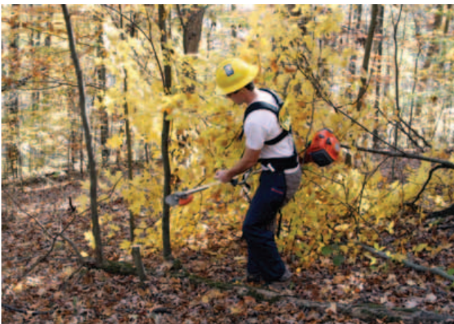
Figure 13. Clearing saws are useful in sapling stands or where there are a large number of small stems to treat. They are much safer and more efficient than chainsaws in these conditions.
